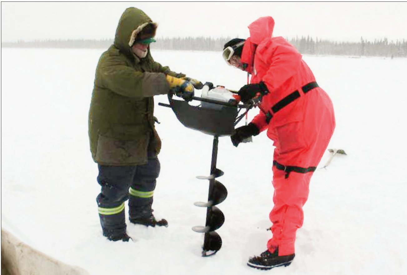
Henry McKay of Fort Resolution, left, and University of Saskatchewan hydrologist Karl Lindenschmidt drill holes in the frozen Slave River to measure ice thickness last winter as part of the initial monitoring work.
